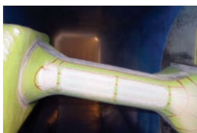
Tunnel ice accretion agreement validating the analytical prediction and test setup
