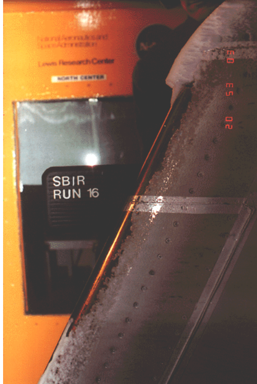
Figure 7: Clean leading edge with a properly controlled heater (Run #16)
