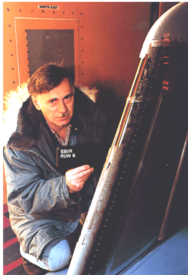
Figure 10: Comparison between heated and unheated sections (Run #6)
