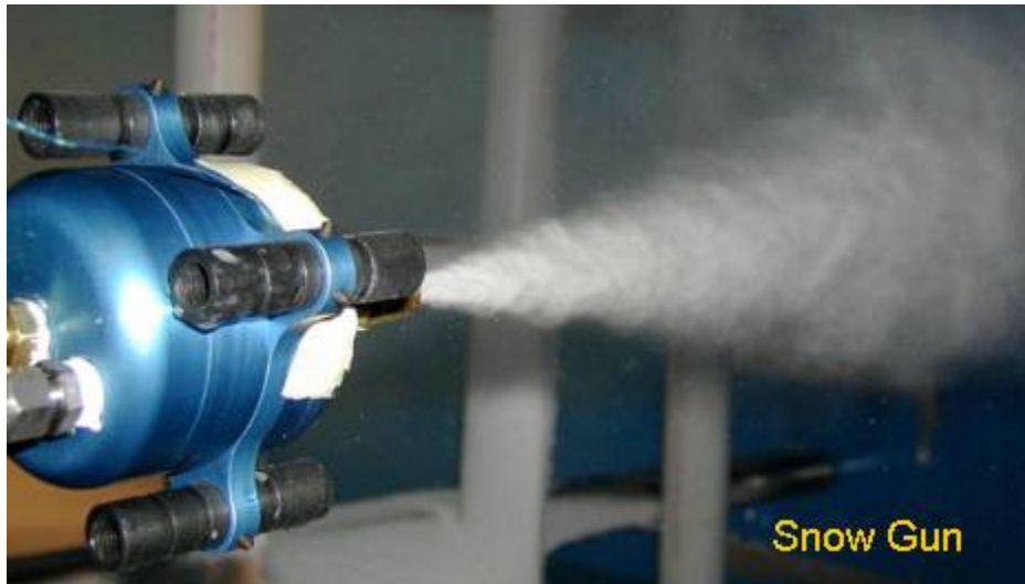
Figure 2: Snow gun in the Cox IWT
