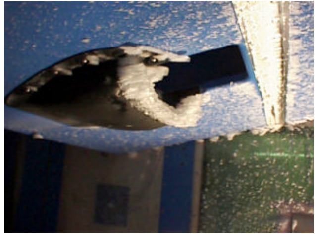
Figure 8: Glaze ice accretion and setup acceptance test for Scoop 1
