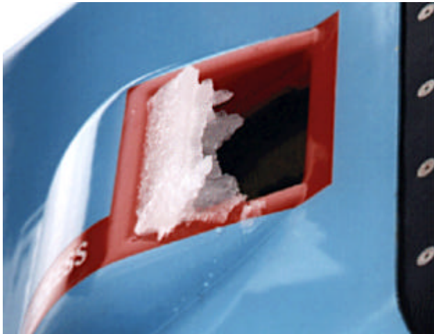
Figure 6: Glaze ice during flight on an earlier version of Scoop 1 (Flight 266)
