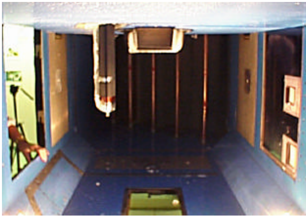
Figure 17: Downstream view of tunnel setup for Scoop 2 with airfoil flow deflector
