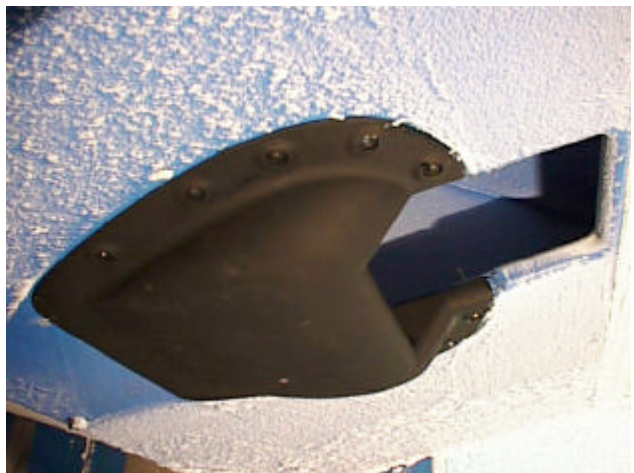
Figure 22: IPS performance during rime and low speed conditions (Scoop 1)
