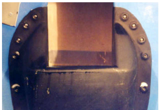
Figure 28: IPS performance during very cold Intermittent Max conditions (Scoop 2)
