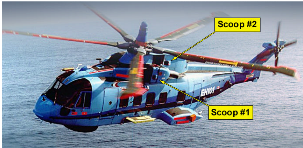
Figure 1: Location of Scoops on the GKN Westland Helicopter (EH101) (Scoop 3 is symmetric to Scoop 1 on Starboard side)
