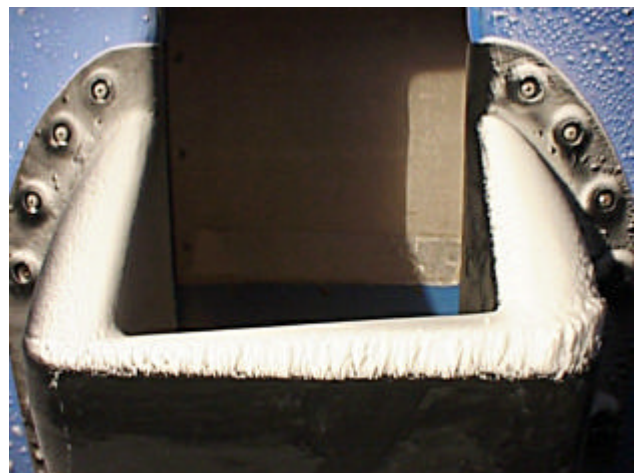
Figure 15: Rime ice on Scoop #2 with full size fairing (opposite effects seen in flight)
