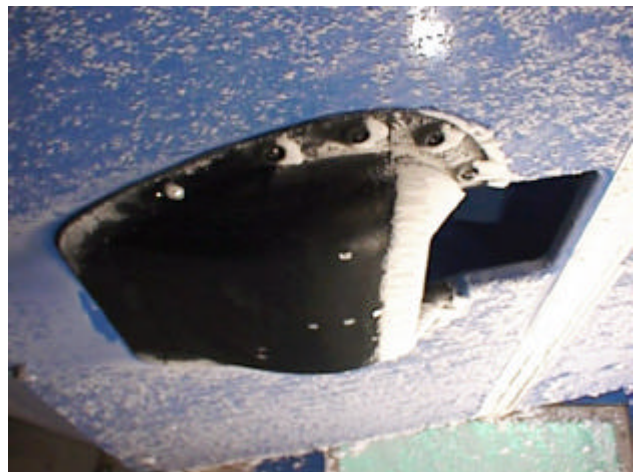
Figure 10: Rime ice accretion and setup acceptance test for Scoop 1
