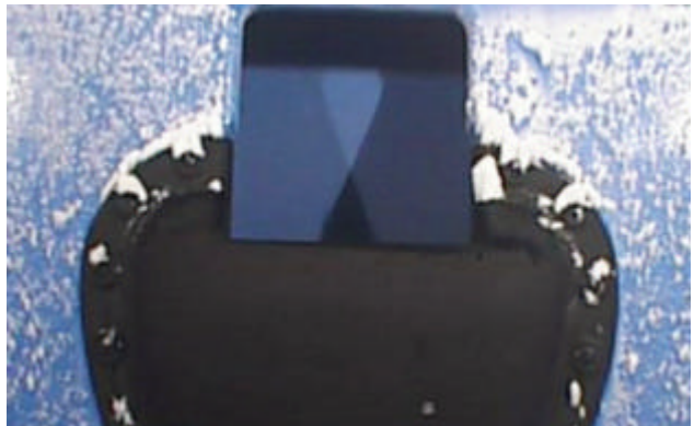
Figure 21: IPS performance in rime icing conditions (Scoop 1)
