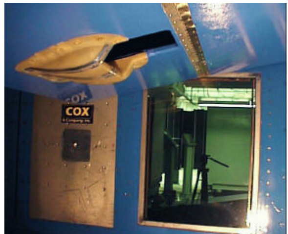
Figure 4: Scoop 1 tunnel setup in Test Section-2
