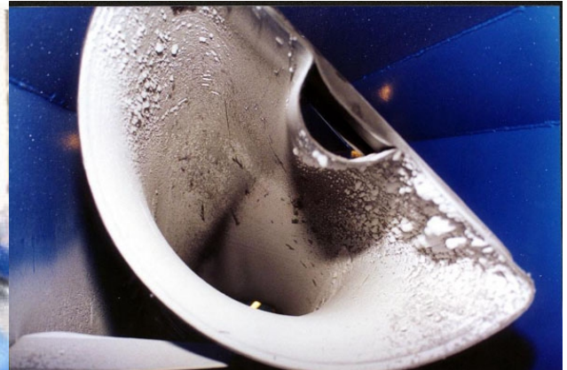
Figure 5: Typical ice accretion in the duct (trailing edge view)
