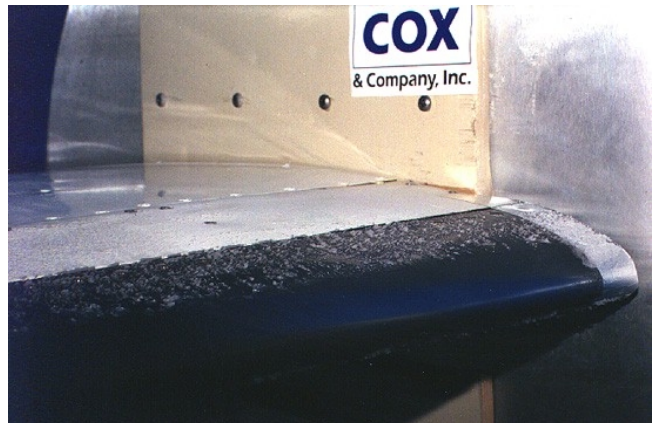
Figure 9: An Ice Protected Horizontal Stabilizer under Testing
