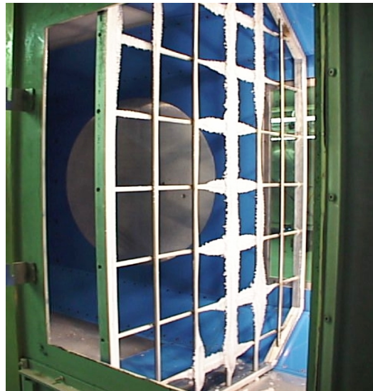
Figure 8: Cloud Uniformity Calibration Grid (one column of nozzles in this case)
